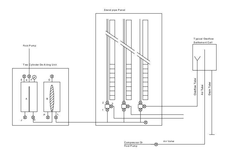
Figure 2: Typical Arrangement for Hydraulic Overflow Settlement Cell With Back Pressure Unit
